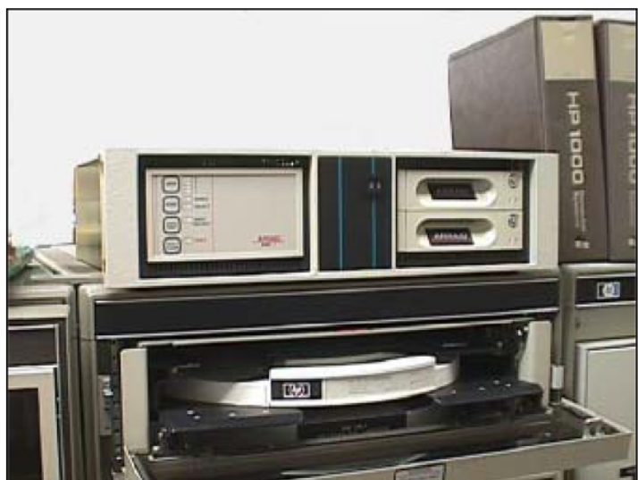
The AEM-6C emulator for the HP 1000 with MAC (Multi-Access Controller) interface includes removable solid state ARRAID Flash Drive (AFD) configured as a hard drive and disk to disk copy/backup to the secondary solid state AFD disk
