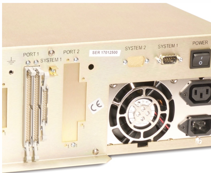
Rear panel of the AEM-6C showing the PC Board Edge “Control” connector and “Data” connector. Connectors are plug-compatible with the original cables.
